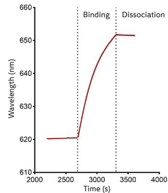
A spectrometer transforms the displacement of the wavelength into a curve that reflects the binding and quantity of the marker in real time.
