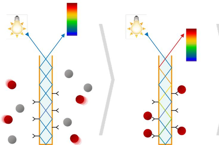
On the gold-coated glass fibre are antibodies that specifically bind a target molecule.
