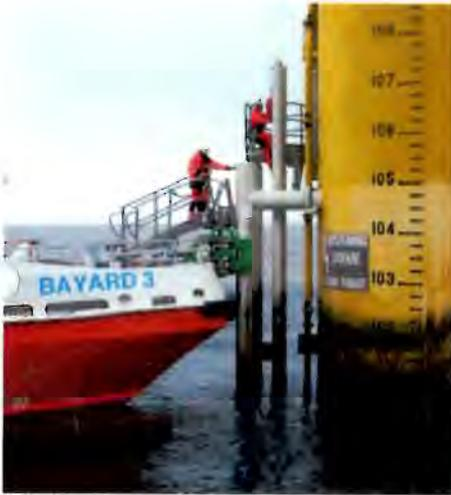
MaXcess is a simple and proven solution to the challenge of providing safer, weather tolerant access in harsh and unpredictable seas. By restraining bow motion while allowing the vessel to roll, pitch and yaw freely, MaXcess is able to extend the wave height limit of personnel transfers for a wide range of vessels.
