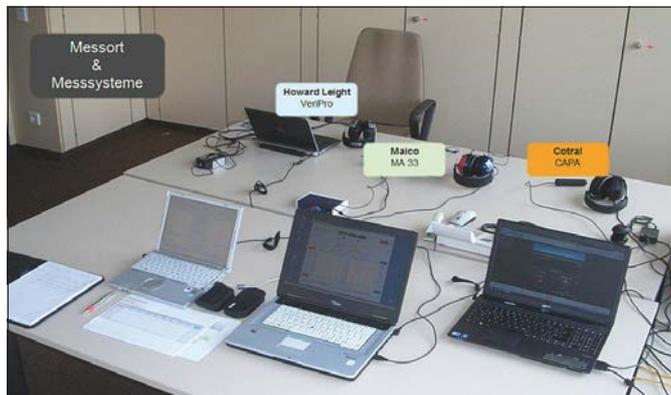
Figure 2 Experimental setup of first study. Each measurement system is controlled by a separate computer.
