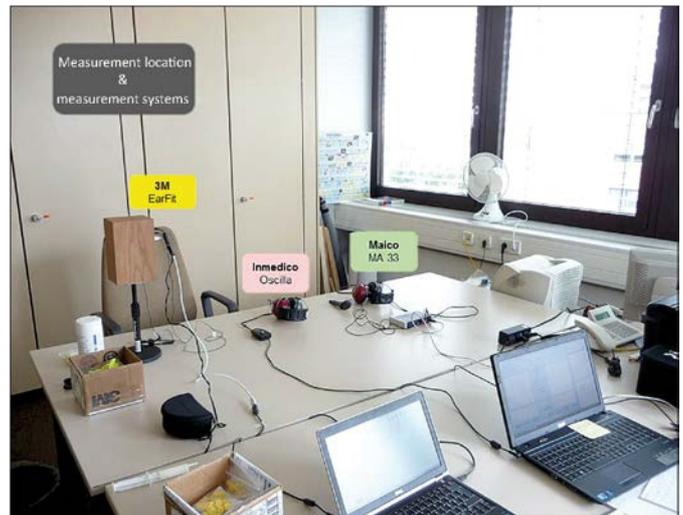
**Figure 4** Experimental setup of the second study. Each measurement system is controlled by a separate computer.
