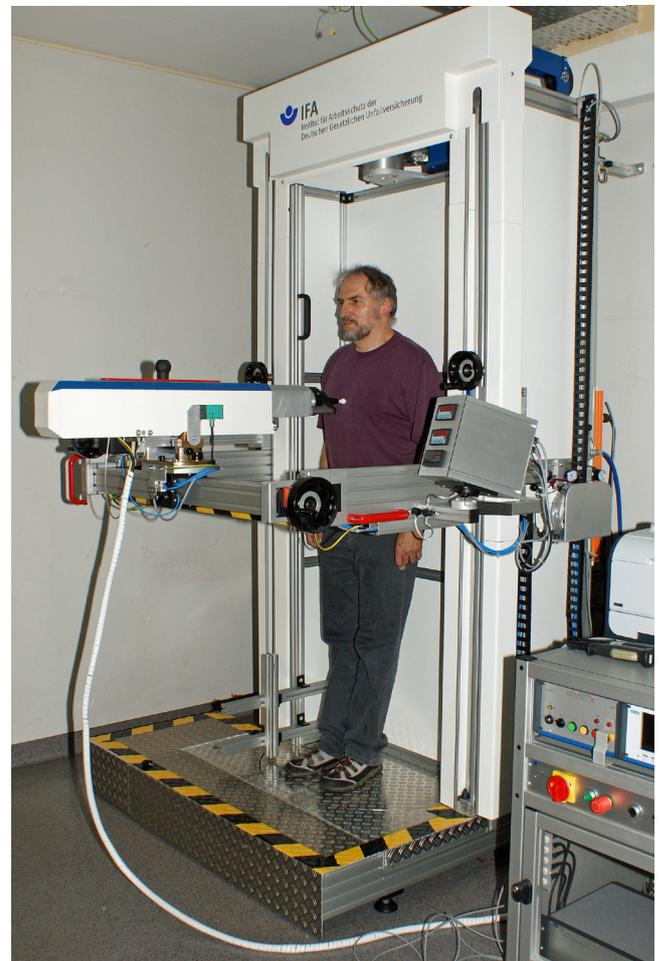
Test facility with algometer
