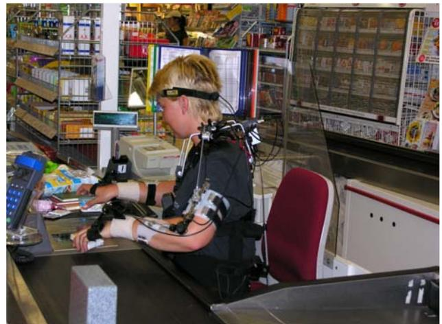
Checkout operator with CUELA measurement system for recording of postures and movements of the shoulders, arms and hands
