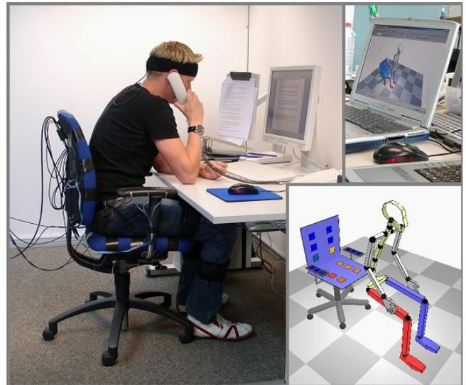
Measurement at a simulated office workplace in a laboratory environment; display in the CUELA software
