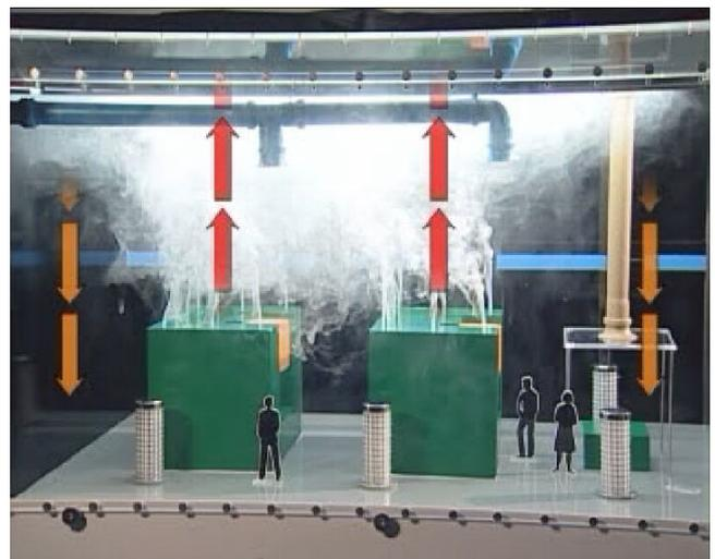
Thermal currents in an area containing sources of heat
