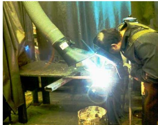
Emission of optical radiation during arc welding
