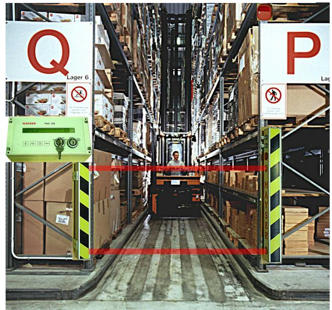
Stationary warning device for securing access to a narrow pathway in a high rack warehouse
