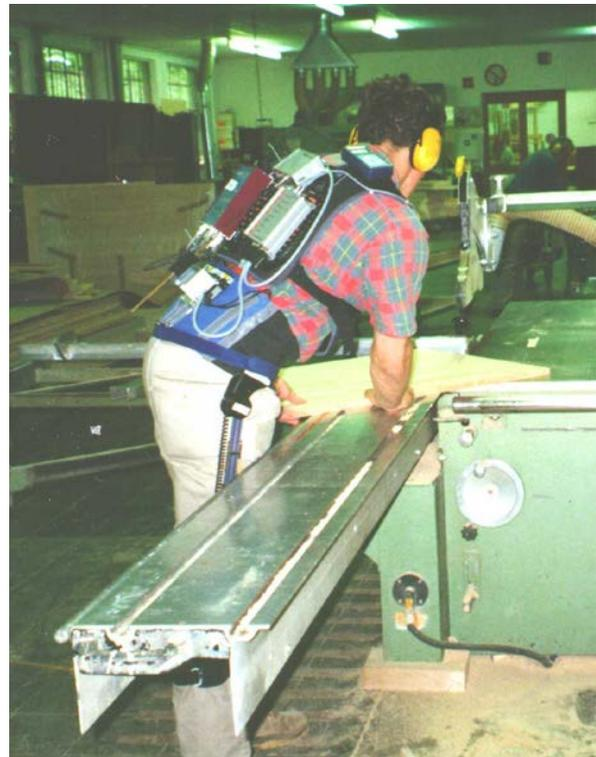
Work with a circular saw; measurement with the CUELA system
