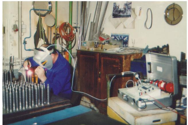
Measurement of ozone exposure during welding work
