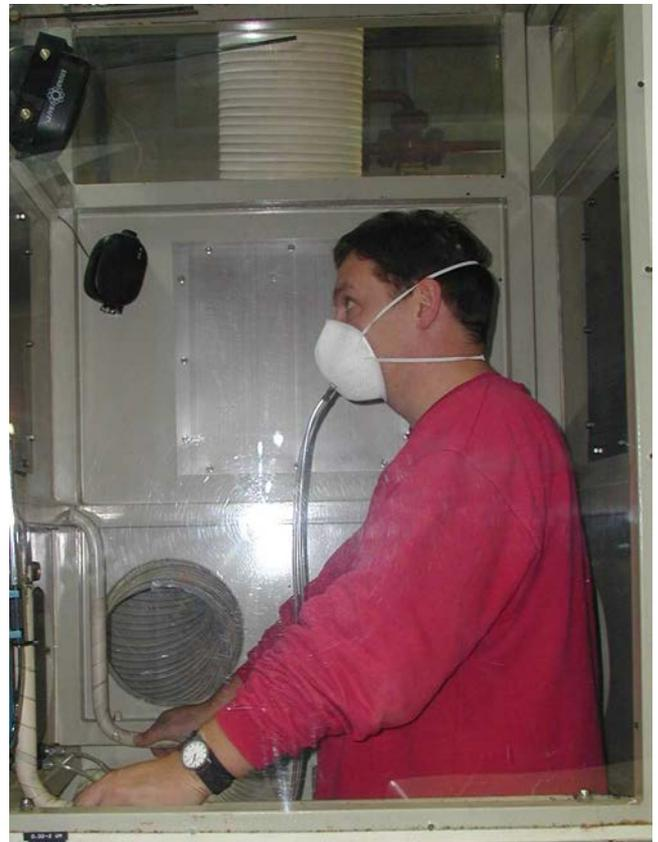
Leakage measurement on a dust mask
