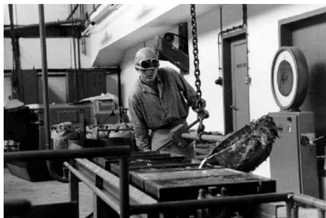
Metal pellets containing cadmium in ingot casting
