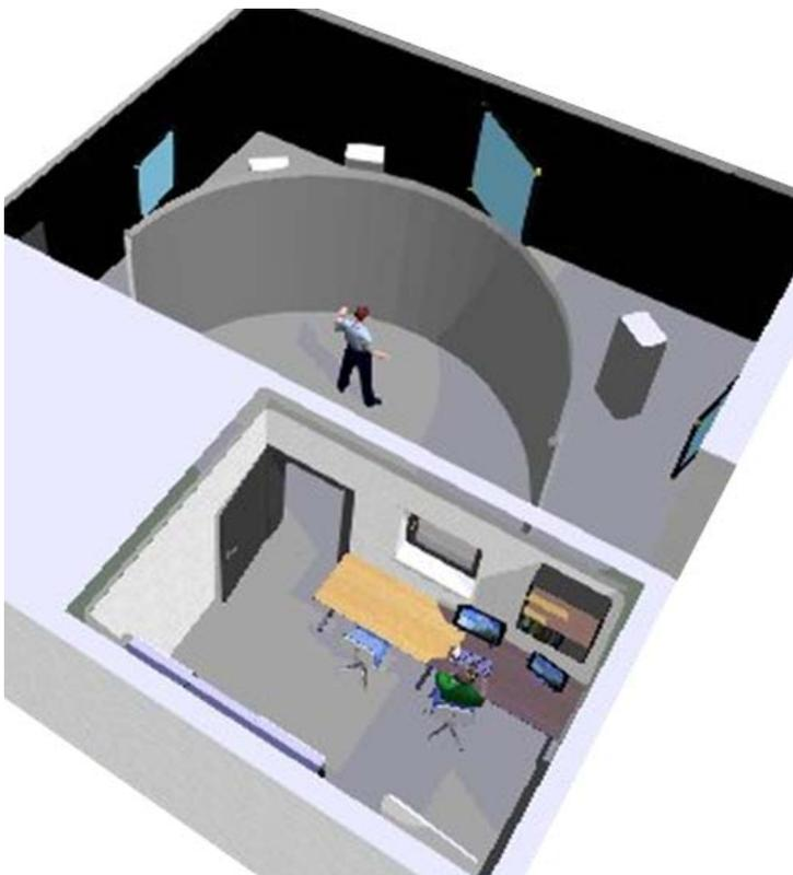
Figure 1: Layout of the SUTAVE laboratory showing VR interaction room, projection wall and rear-projection equipment, and the room in front of the projection wall from which virtual work scenarios are controlled
