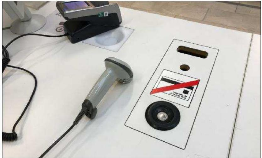
Figure 2: Magnetic hard label remover
