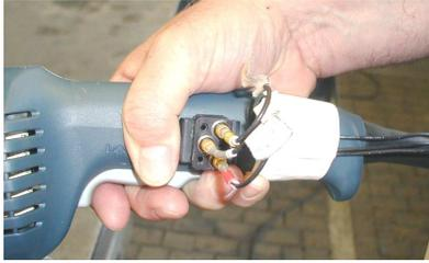
Figure 4 - Main handle of the angle grinder with integrated switch
