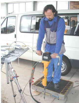
Figure 3 - Use of a reference measurement chain for examination of the measurement system
