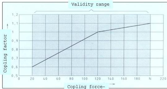
Figure 1 - Influence of the coupling forces to DIN 45679
