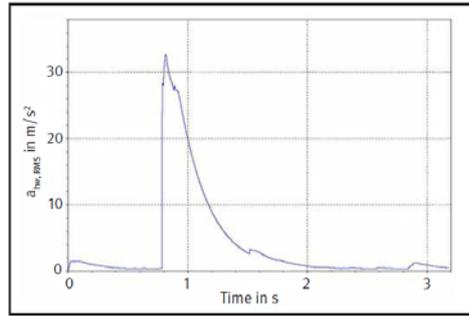
Figure 3: Time characteristic of the flat<sub>h</sub>-weighted running root-mean-square value
