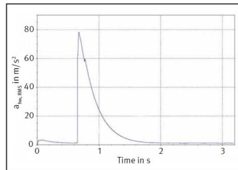
Figure 9: Time characteristic of the flat<sub>h</sub>-weighted running root-mean-square value
