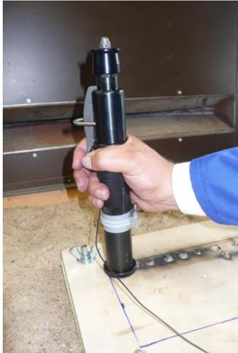
Figure 7: Performance of testing with cattle stunning apparatus
