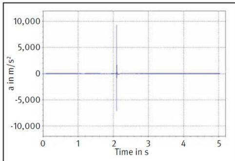
Figure 11: Time characteristic of the  $flat_h$ -weighted acceleration
