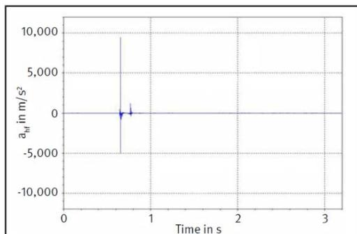
Figure 8: Time characteristic of the flat<sub>h</sub>-weighted acceleration
