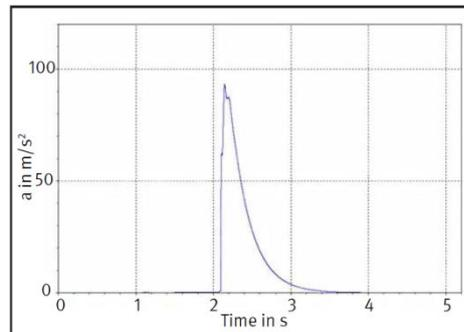
Figure 12: Time characteristic of the  $flat_h$ -weighted running root-mean-square value
