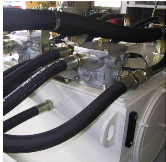
**Figure 5:** Return line filters on a hydraulic tank
