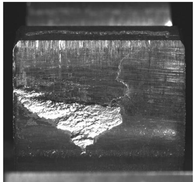
**Figure 8:** Tooth flank damage
