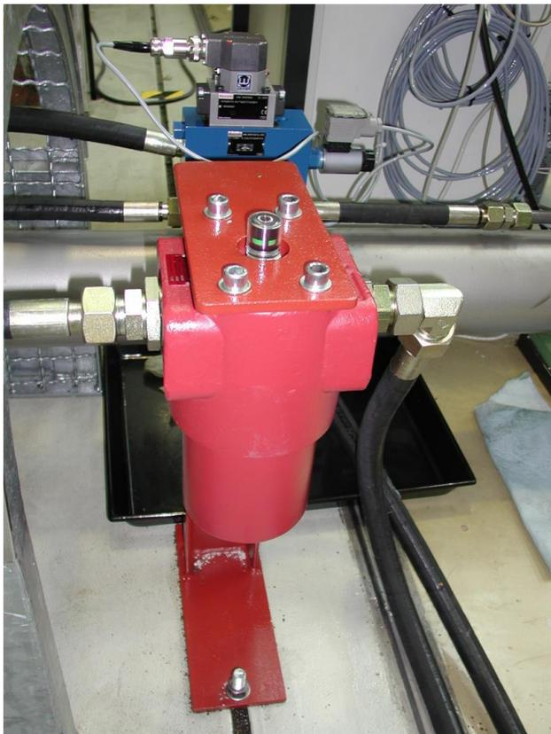
Figure 1: Filter on a hydraulic power unit
