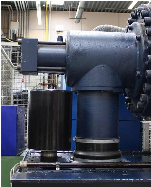
**Figure 7:** Breather filter on pedestal
