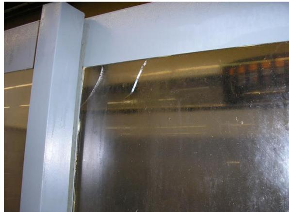
Figure A6: Cracks starting from the panel edge in embrittled polycarbonate panel
