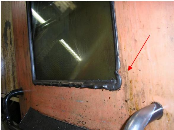
Figure A5: Swelled panel sealing due to metalworking fluid. The lateral tightness to the polycarbonate panel edges is no longer existent (applies also to cracked panel sealings).
